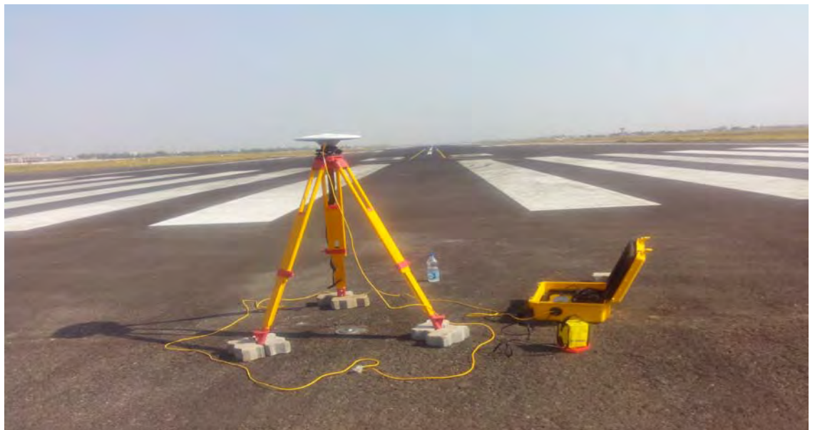
GPS Observation at Ahmadabad Airport for providing Control point.
